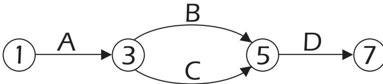
**Fig. 10.8** An incorrect network diagram for activities A, B, C and D.
