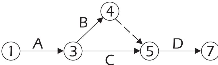
**Fig. 10.9** A correct network representing activities A, B, C and D after dummy activity 4-5 has been introduced.
