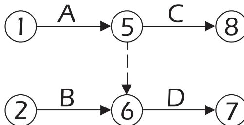
**Fig. 10.7** Network for the problem showing the dummy activity 5-6.
